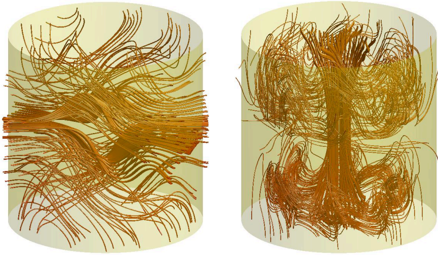
Figure 7: Geometry of the dynamo mode obtained by kinematic numerical simulations: (left) an equatorial dipole is generated by the mean flow alone. (Right) When a non axisymmetric velocity component is taken into account, an axial dipole is generated (Figures from Gissinger 2009).
